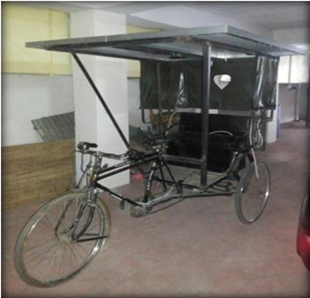
Fig. 4. The rickshaw with the PV array installed
